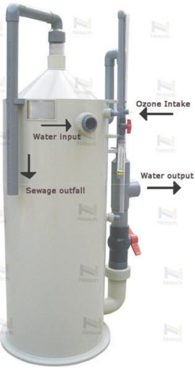
The protein skimmer can be used to reduce the physical and chemical gels. It uses the role of adsorption of surface tension of the bubble to enrichment and separation organic, removal the colloidal suspension, cellulose, protein, bait and faeces and other organics in the wastewater. Meanwhile, the protein separator can be used as an ozone mixing tower, which can separate protein and use ozone to do the disinfections.
